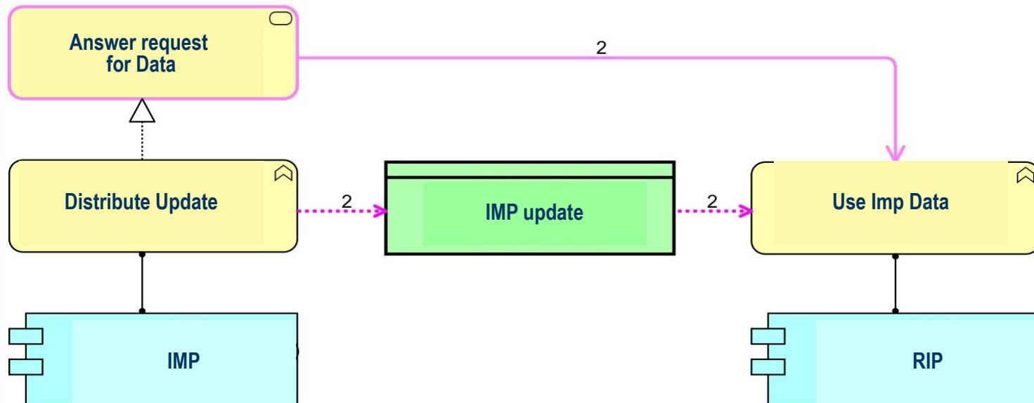
GW shows show data in flow as a **data object** passing from a **function** to a function
