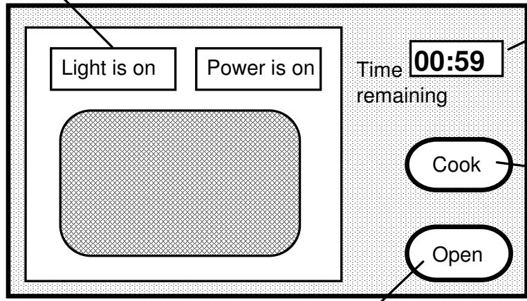
Open the door while the power is off - the light comes on.
