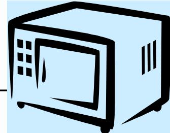
When the oven timer reaches zero, it turns off the power tube, turns off the light and sounds the beeper to tell you the food is ready.
